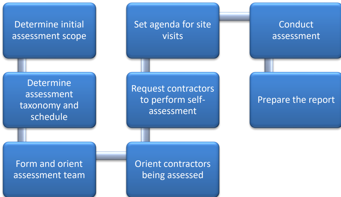
Figure 4-1 – Sample Process Flow for Conducting MRL Assessments
